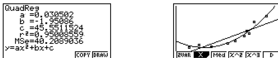
Figure 11. The quadratic function model y = 0.03x^2 - 1.95x + 45.5 fits the data
