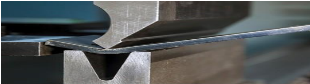
Figure 3: Fabrication Process of a Metal Channel
